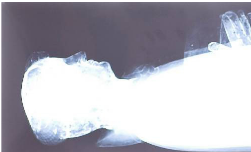
Figure 7: over-exposed digital photography of a film radiography
