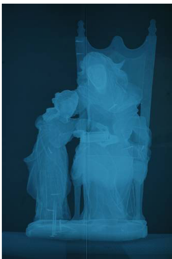
Figure 1 - Example of an well exposed radiography of an wooden sculpture, (“St. a Ana e N. a Sr. a ”, possibly from XVIII century) digitalized with a DSLR camera (Nikon D70), without digital treatment (only converted from RAW to JPG file).
