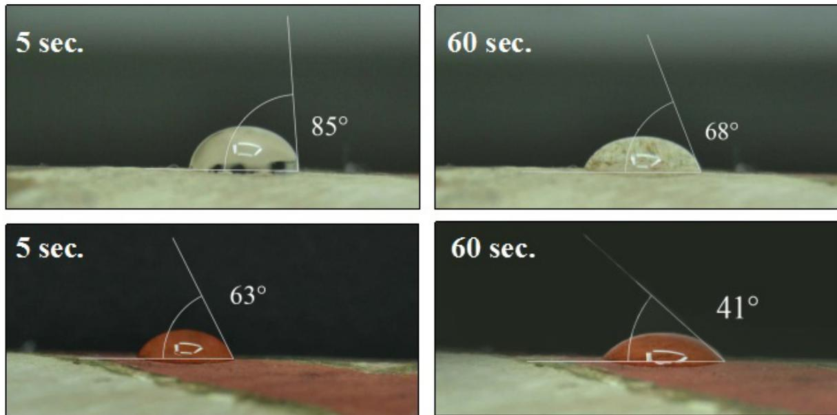
**Figure 6** – Time evolution of white (top) and red (bottom) paint contact angle.
