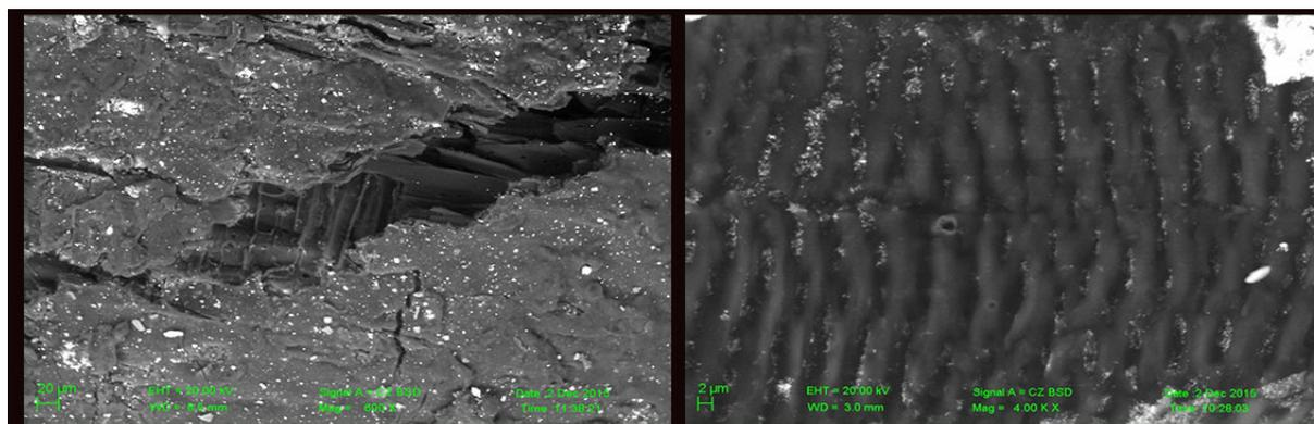
**Figure 2** – SEM images of the *dyera costulata* wooden substrate: the low magnification micrograph (left) shows the highly irregular surface, at high magnification (right) the porous structure of the wood is highlighted.
