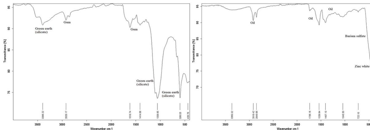
**Figure 3** – FTIR spectroscopy of the green pigment sample - green earth - with gum binder (left) and of the white pigment sample - zinc oxide - with oil binder (right).
